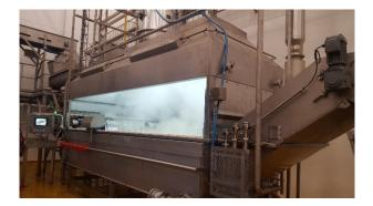
Fabcon Food Systems builds a range of batch fryers for hand cooked, hard bite artisan style potato crisps/chips for up to 300 kg/hr of finished product.
